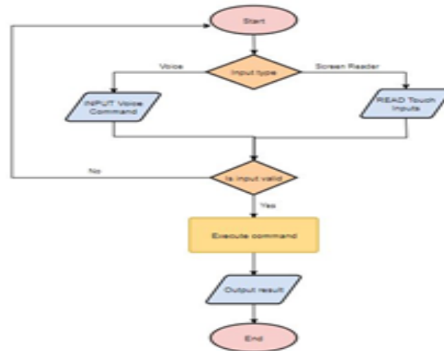
Figure 1: Activity Diagram for proposed system
