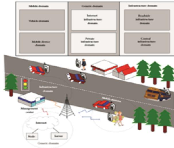
Figure 3: Vanet Main Components Architecture.
